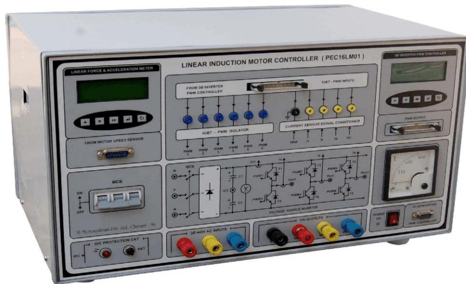
Linear Induction Motor controller
